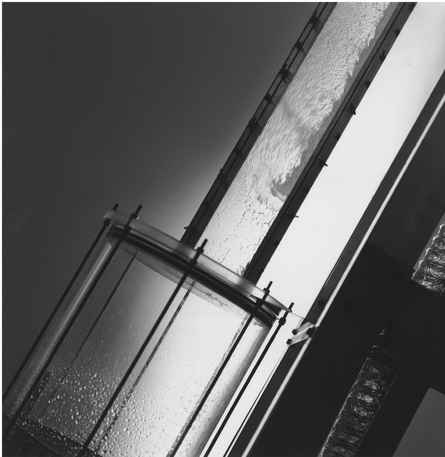
Fig. 4. Air–water flow pattern inside the 100 mm duct inclined at 60^\circ to the horizontal. V_G = 19 m/s, V_L = 9.2 \times 10^{-3} m/s, Re_G = 22300 , Fr_{HG} = 0.41 .
